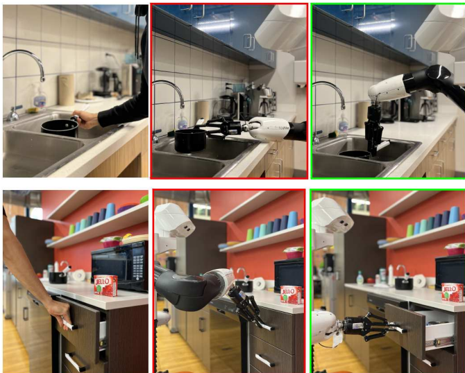
Fig. 5. Grasping mode adaptation. Two examples ( top and bottom rows ) of SAFEMIMIC’s grasping mode adaptation. Left column : human demonstrated grasp. Middle column : robot failing when attempting the task by matching the human grasp. Right column : robot succeeding in the task through SAFEMIMIC’s grasp adaptation. In 6 out of 7 tasks, SAFEMIMIC’s grasp adaptation is critical to overcome human-robot embodiment differences and successfully imitate the demonstration.
