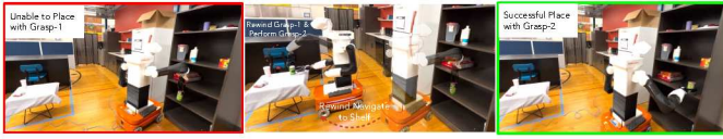
Fig. 11. Backtracking actions in SAFEMIMIC. Example sequence of backtracking behavior in Shelving task. When no safe samples are available, or when a segment exploration ends without success, SAFEMIMIC backtracks to previous states by undoing the last actions, possibly stepping back to explore a different grasping mode. This simple but effective mechanism enables autonomous exploration and adaptation of human motion for multi-step mobile manipulation tasks with SAFEMIMIC.
