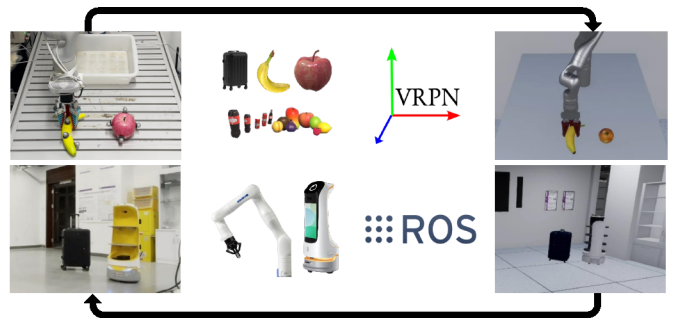
Fig. 2: Virtual-Real Data Synchronization Framework. The central demonstrates the synchronization of object pose and robot motion through VRPN and ROS. The left and right parts depict the virtual simulation environment and physical real world scene, respectively.
