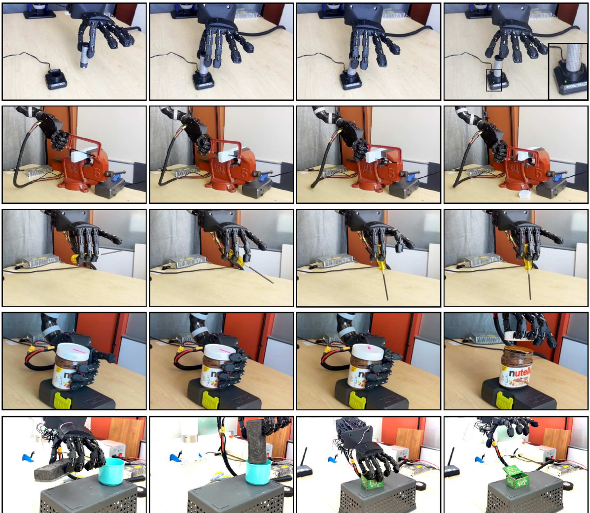
Fig. 10: Teleoperated tasks made possible with RUKA. The top three rows showcase teleoperation of in-hand grasping tasks, while the remaining rows demonstrate arm-and-hand teleoperated tasks.
