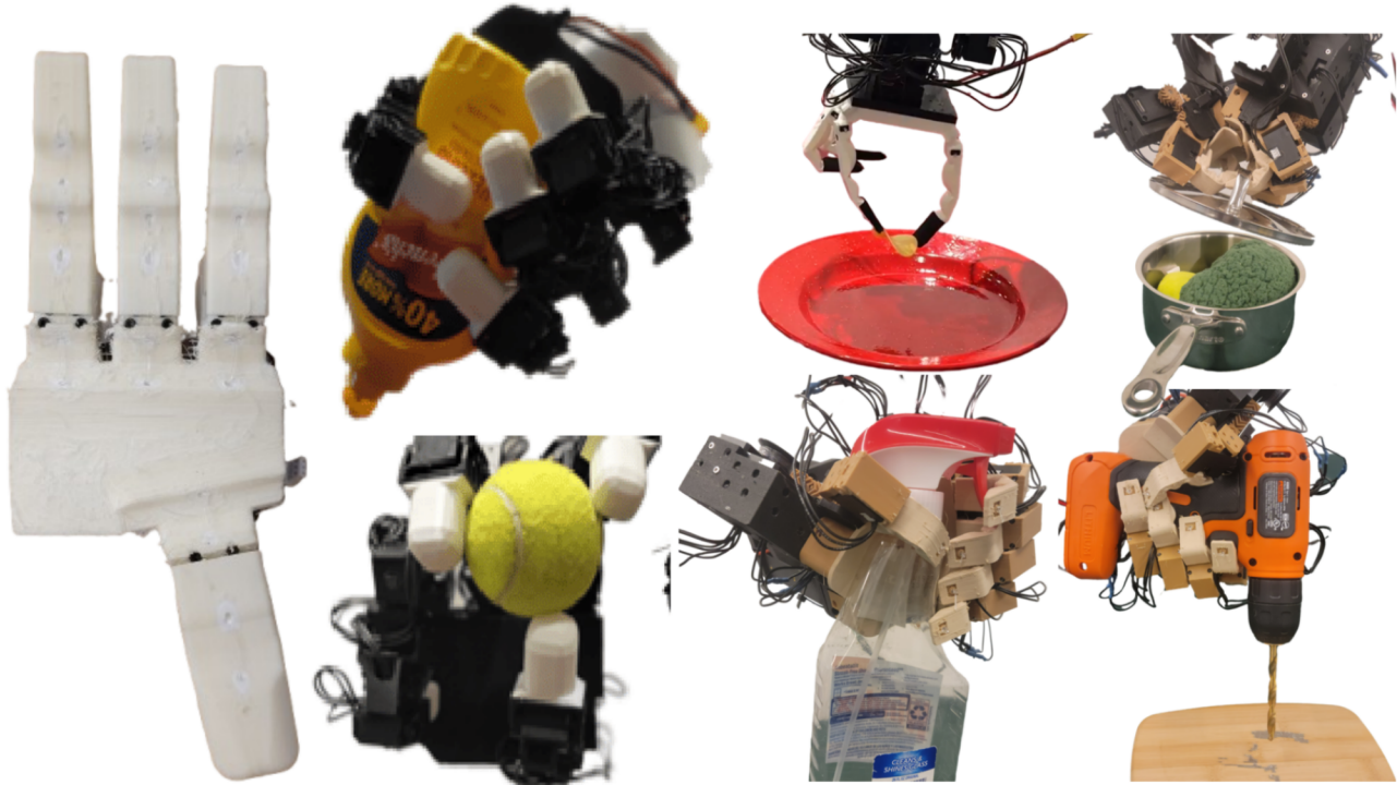
Fig. 1: Our demonstration will feature four different low-cost, open-source robotic hand designs, including a new model introduced in this paper, LEAP Hand V2. (left) These hands are highly dexterous, easy to build, durable, and affordable. We also provide a suite of open-source software tools, including motion capture teleoperation, human video-based learning, and reinforcement learning capabilities. Building on our successful demonstrations at RSS 2023 and 2024, we aim to further highlight the potential of low-cost, open-source robotic hands and strengthen our open-source robot hand community at RSS 2025. Please visit our website at https://leaphand.com for more details.
