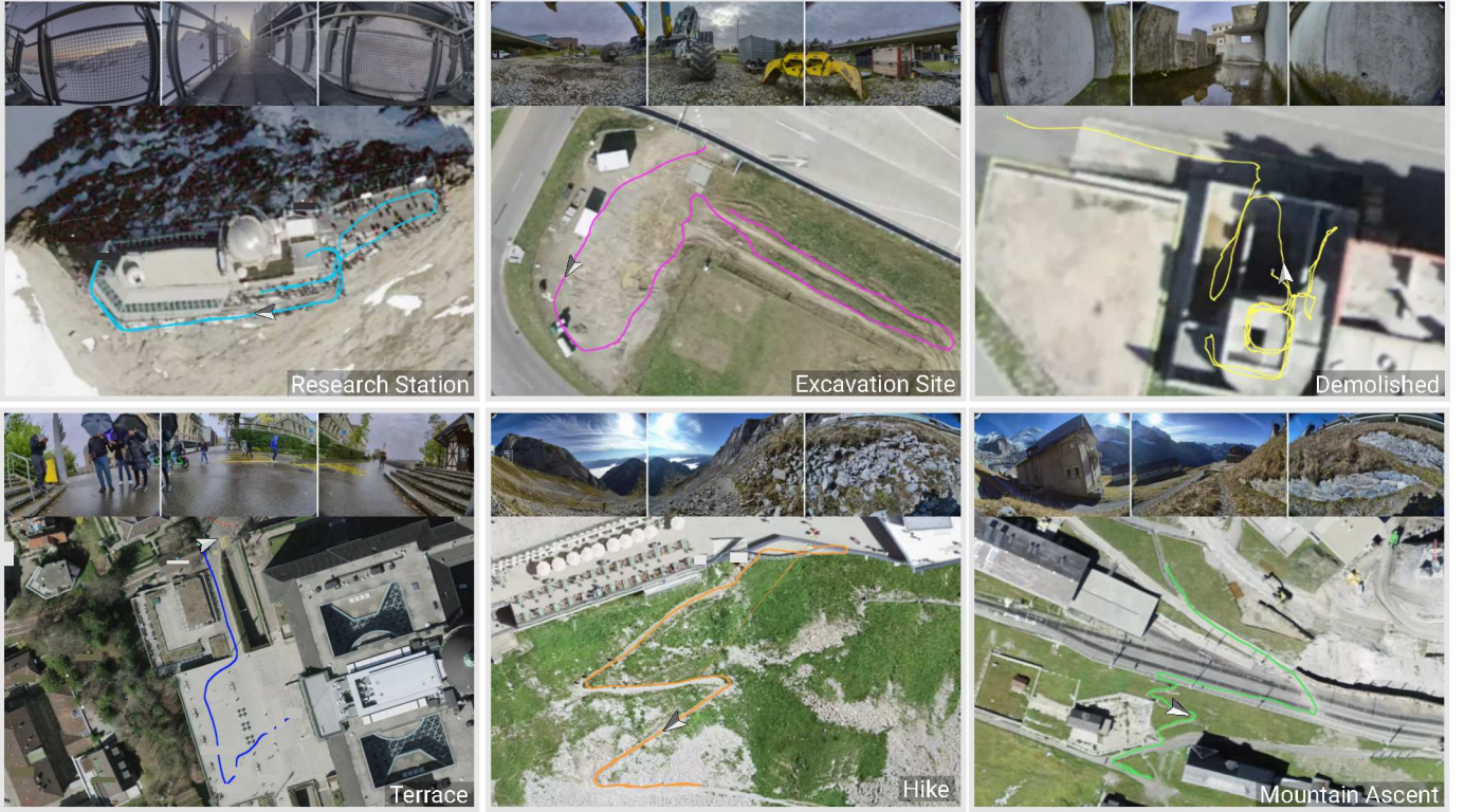
Fig. 3: Subset of the GrandTour Datasets Overview: (top-row) left, front, and right HDR camera images; (bottom-row) satellite image with projected GNSS path and camera image viewpoint; The warehouse dataset is not displayed.
