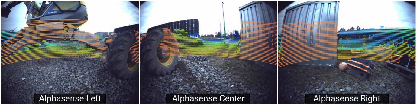
Fig. 21: Overlay of the LiDAR point cloud while moving forward at 1 \text{ m s}^{-1} , showcasing the consistency of the sensor calibration and the motion undistortion of the point cloud.
