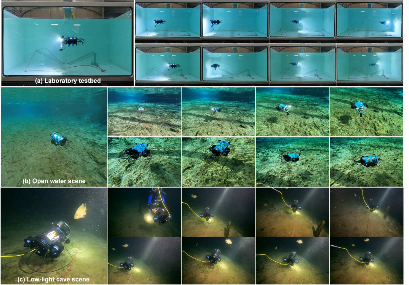
Fig. 15: A few snapshots from our field trials for caveline tracking and following experiments with CavePI are shown. The setups include: (a) rectangular loops and slopes in a water tank; (b) irregular shapes in Spring riverine water, and (c) low-light underwater cave scenarios (note that the tether is only for safety and easy recovery). Images are best viewed digitally at 2\times zoom; full video demonstration is submitted in the supplementary files; also available online at: https://youtu.be/9BPpB1nu98E .
