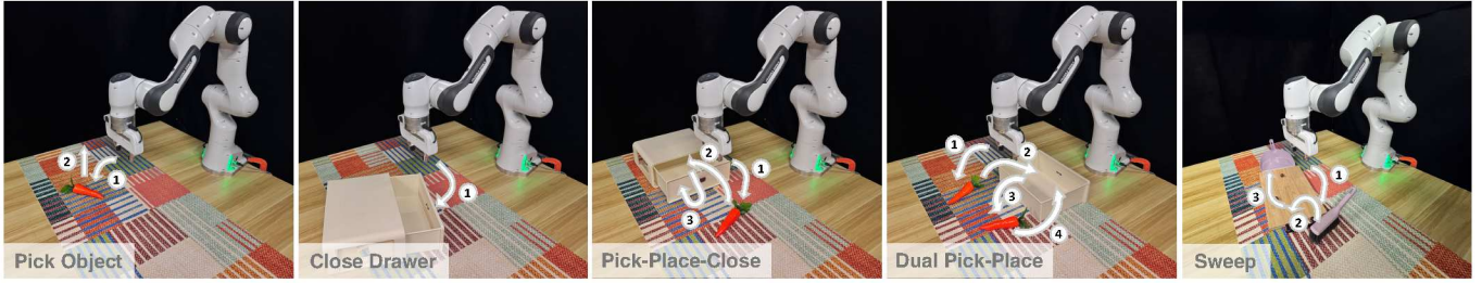
Fig. 6: Task illustration. We design five manipulation tasks for real-world evaluation: Pick Object , Close Drawer , Pick-Place-Close , Dual Pick-Place and Sweep , whose details are elaborated in Sec. V-A.
