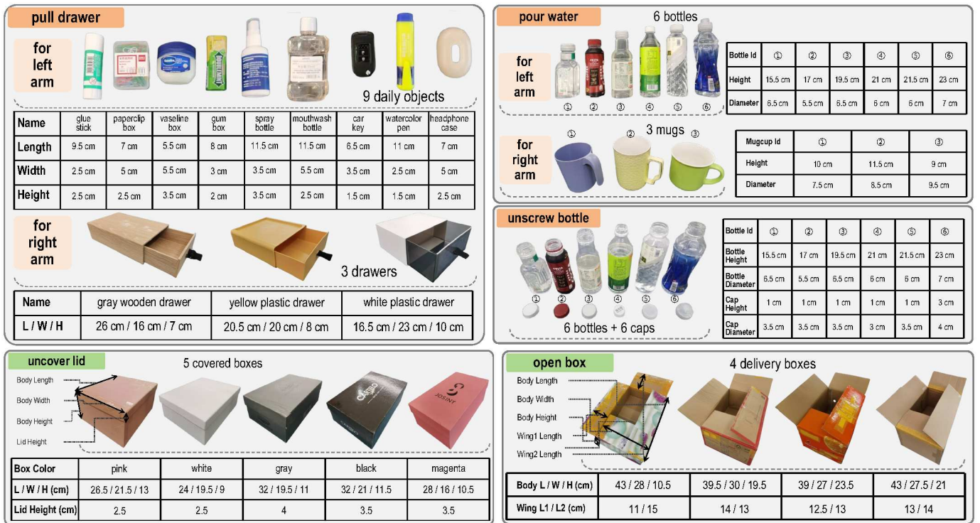
Fig. 10: We collected a variety of manipulated objects in instance-level for each of five bimanual tasks to improve and verify the generalizability of trained policies. All of these objects are from everyday life, not intentionally customized. We also collect the detailed size information in centimeter-level for all related objects. Best to view after zooming in.
