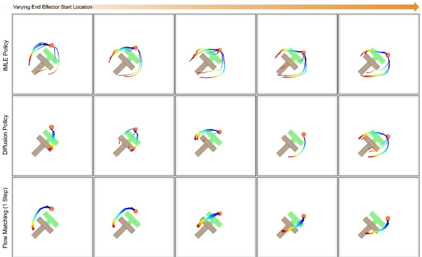
Fig. 2: Qualitative Analysis of Mode Capturing Performance. Illustrating the open-loop trajectories generated by different methods (rows) for varying initial end-effector positions (columns) in the Push-T task, where multiple trajectories were generated for each condition using different random seeds. The goal is to push the T-shaped block from its initial position to align with the target (green). The dataset exhibits multi-modality, with human demonstrations performing the task through various modes of behaviour, for example going either left or right to get to the opposite side. IMLE Policy successfully captures all modes without collapsing or biasing, maintaining trajectory diversity even in underrepresented modes. In contrast, Diffusion Policy tends to bias towards one mode when close to an edge, showing sensitivity to initial conditions, while Flow Matching collapses modes, producing averaged and unimodal trajectories.
