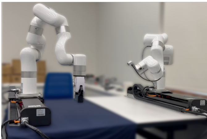
Fig. 7: The 17-DOF robotic system for real-world experiments aligns with the MVS simulation environments. It includes two xArm7 mounted on linear motors, with camera and gripper attached to each end effectors.
