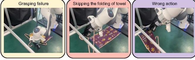
Fig. 16: Classical failure modes of baselines in Hang Towel , including grasping failure, skipping the folding of towel, and wrong action (directly putting the towel onto the rack without the hanger).
