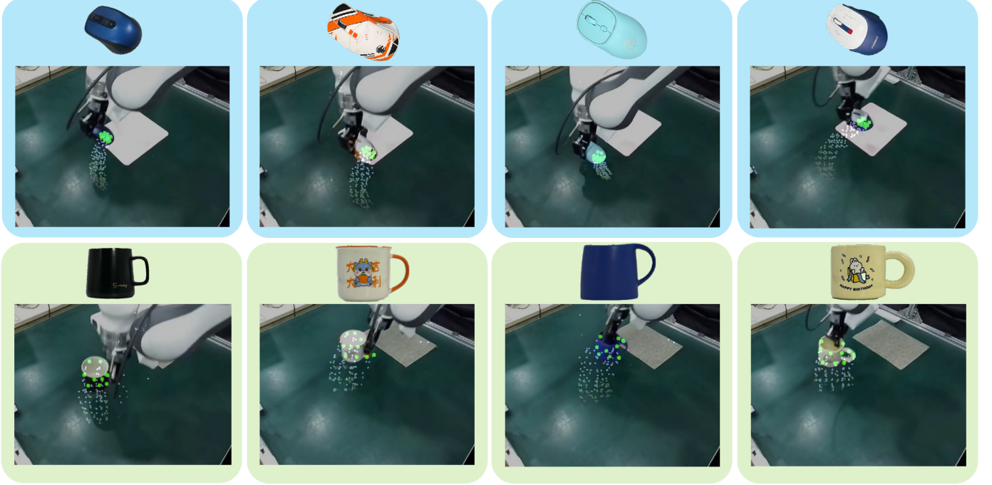
Fig. 13: Movement of semantic keypoints on different objects in SKIL. Green points represent the current keypoints, and the white flows show their previous trajectories. Temporal consistency is maintained across objects within the same category.
