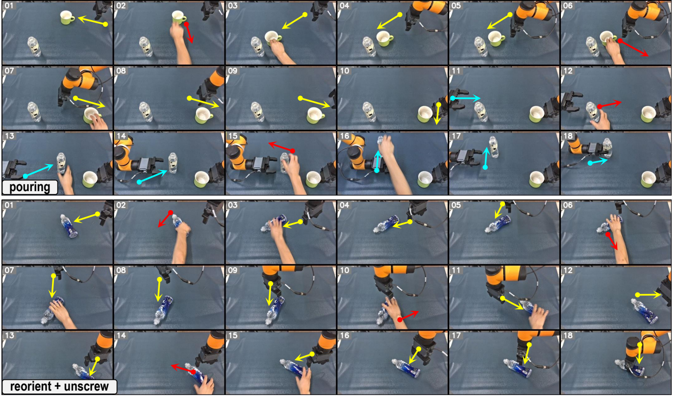
Fig. 17: Qualitative examples of applying dynamic interferences during the pre-grasping execution. From top to bottom, they are segments of the dynamic closed-loop grasping phase of tasks pouring and reorient+unscrew , where each object is manually disturbed from one to three times. The red arrow indicates the direction of the manually moved object (interfering). The cyan arrow and yellow arrow indicate the movement direction of the left and right robotic arms (chasing), respectively.
