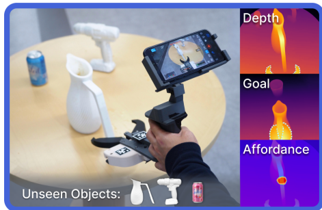
Fig. 1. UMI-Underwater. We address data-collection and generalization bottlenecks in underwater manipulation by pairing autonomous, self-supervised data collection with a zero-shot, depth-based affordance predictor that transfers directly from land to water.
