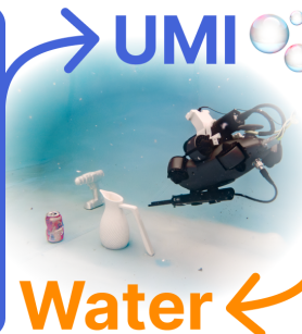
Fig. 1. UMI-Underwater. We address data-collection and generalization bottlenecks in underwater manipulation by pairing autonomous, self-supervised data collection with a zero-shot, depth-based affordance predictor that transfers directly from land to water.
