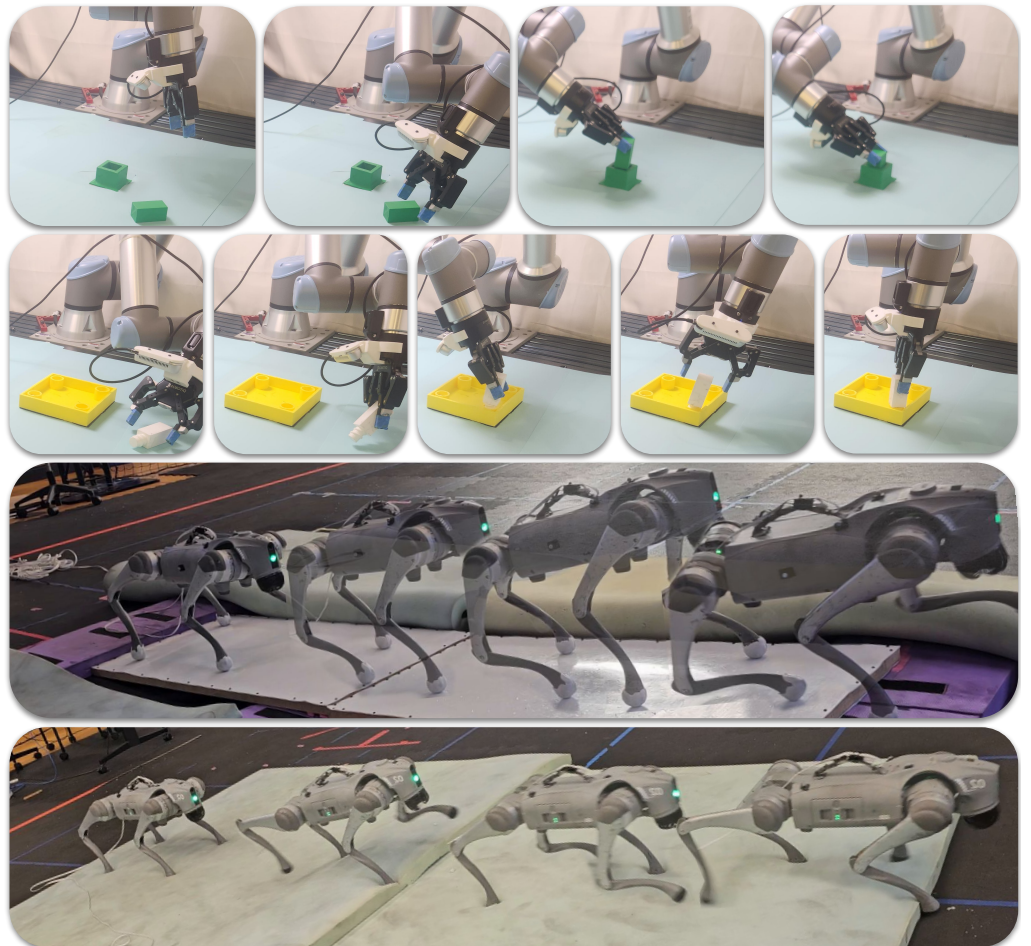
Fig. 1: Failures of zero-shot sim-to-real policies (left). Our framework SimDist rapidly overcomes the dynamics gap and improves performance with minimal real-world interaction. We demonstrate substantial gains in task execution on both precise manipulation and quadrupedal locomotion tasks with only 15-30 minutes of real-world data, substantially outperforming baselines.
