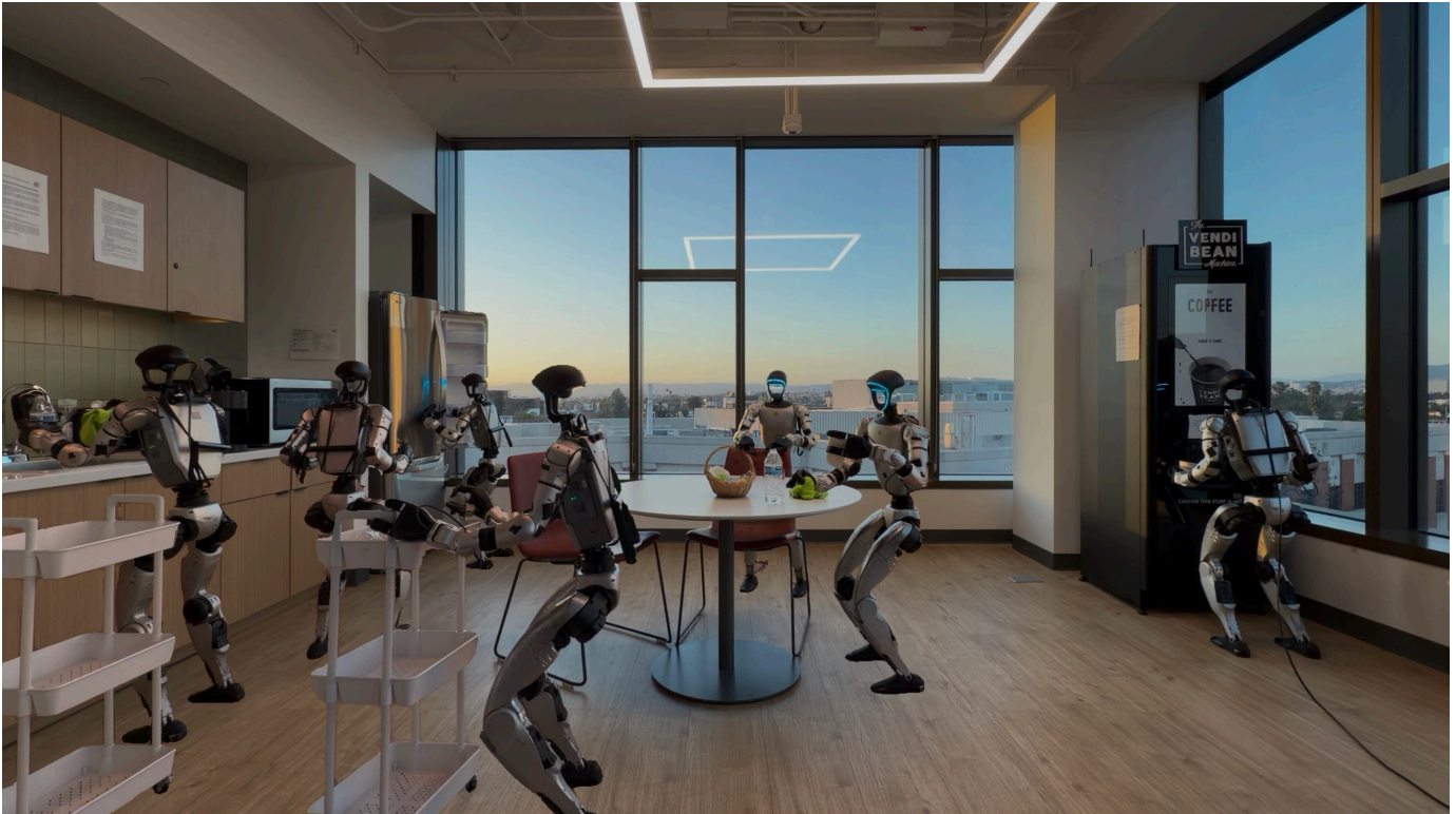
Fig. 1: Humanoid Loco-Manipulation. \Psi_0 performs diverse loco-manipulation tasks in a pantry, including taking a cup from the coffee machine, pushing a cart, wiping the table, grasping a bottle and placing it in the sink, and pushing the fridge door.
