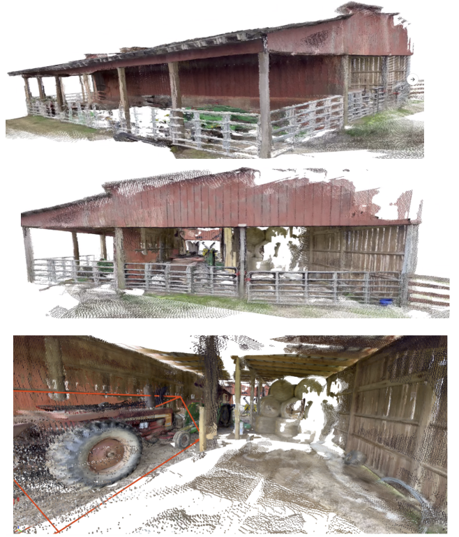
Fig. 9. VGGT-SLAM 2.0 reconstruction of a 4200 square foot barn with 34 submaps of size 16 frames using images captured from an iPhone. An example open-set query detecting a tractor inside the barn with the query “large tractor” is shown in the bottom figure.
