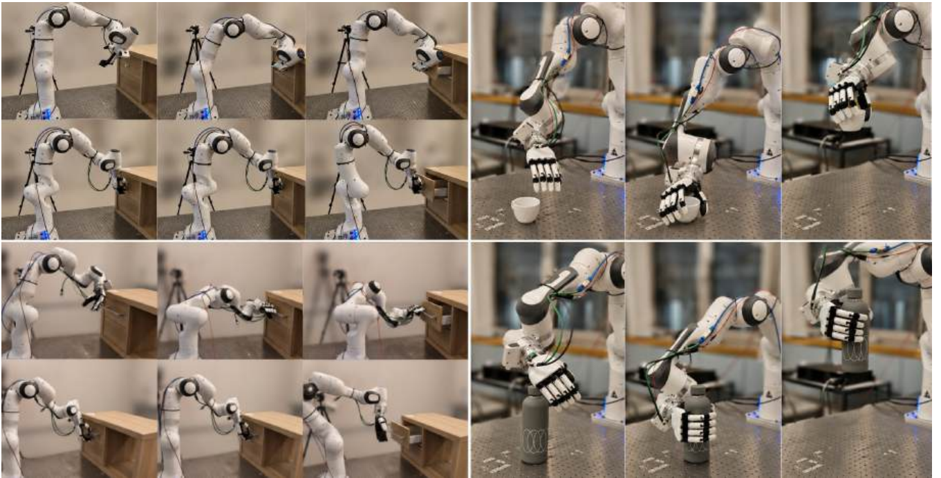
Fig. 9: Real-world cabinet-handle rollout. We sample handle grasps from a point-cloud-conditioned diffusion model trained on refined grasp distributions and then plan collision-aware trajectories using cuRobo. The trajectories are executed on a Franka Panda arm equipped with a dexterous hand. Three executions across different grasp modes and approach directions demonstrate successful sim-to-real transfer in contact-rich manipulation.
