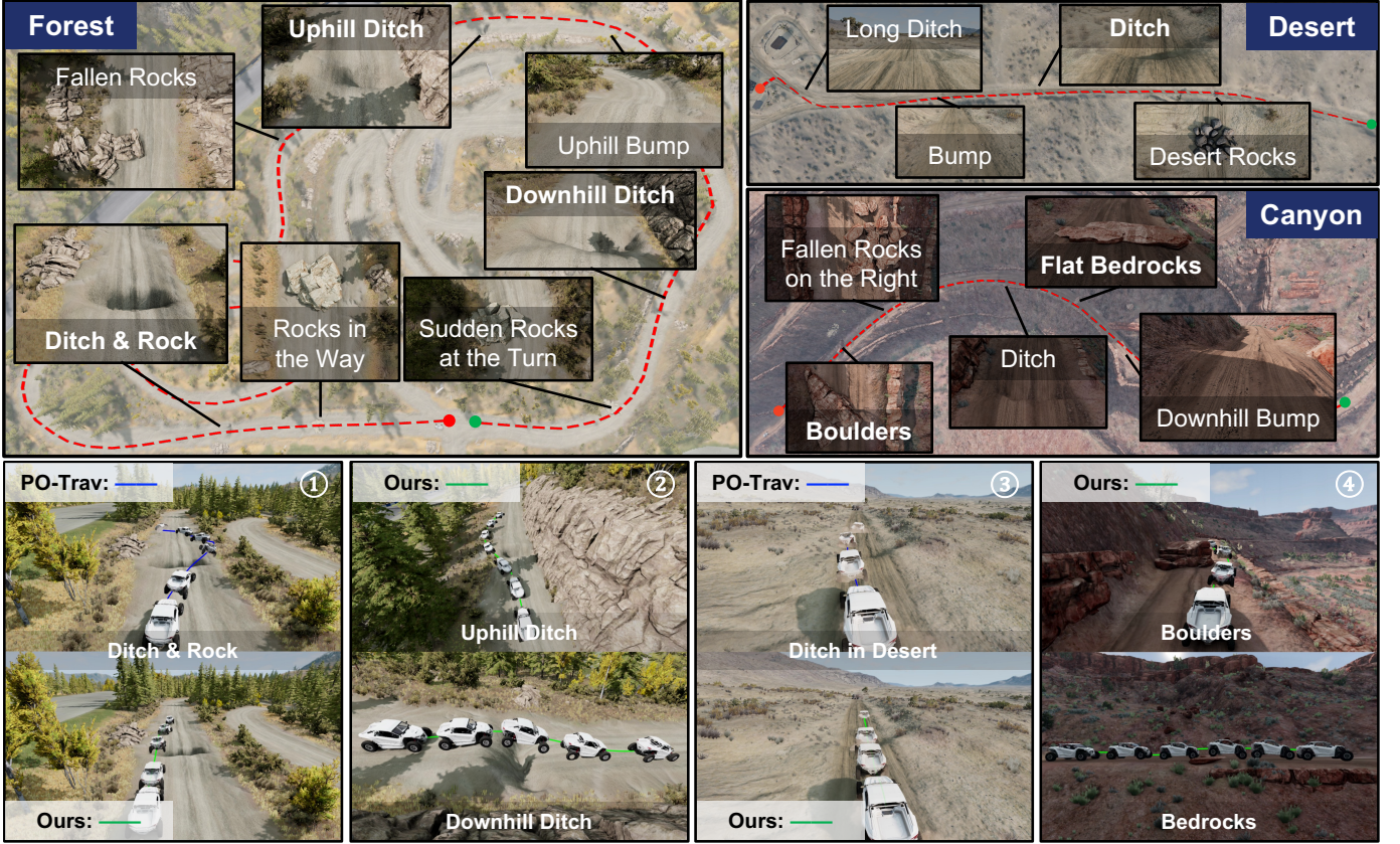
Fig. 6: Simulation maps and qualitative results for the long-range navigation task. The top row shows three modified maps with introduced obstacles blocking the routes. The bottom row presents vehicle trajectories under MAT and the PO-Trav that exhibit distinct behavioral differences, with the corresponding obstacles highlighted in bold on the maps.
