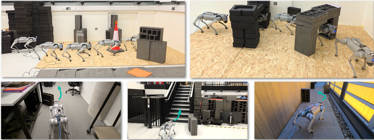
Fig. 1: Real-world demonstrations of SanD-Planner. The proposed algorithm enables the robot to traverse cluttered environments with tight clearance, including navigating narrow passages, avoiding obstacles, and climbing stairs.
