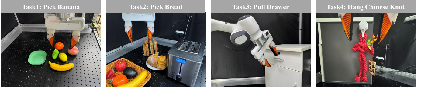
Fig. 3: Overview of real-world experimental tasks: Pick & Place (Banana, Bread), Pull Drawer, and Hang Chinese Knot.
