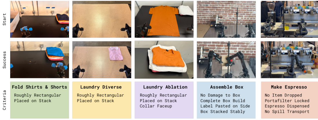
Fig. 5: Evaluation tasks and success criteria. We evaluate three laundry variants, box assembly, and making espresso drinks. For each rollout, human annotators assess task completion using the task-specific quality criteria shown here, such as fold quality and placement for laundry or damage and stability of stacking for box assembly. These criteria are aggregated into a binary success label for reporting success rate.
