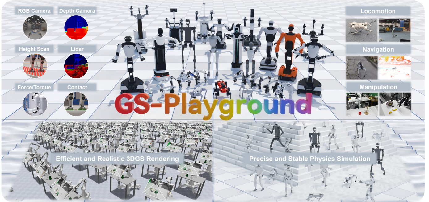
Fig. 1: GS-Playground Overview. It integrates photorealistic 3D Gaussian Splatting with high-performance parallel physics, achieving over 10^4 aggregate FPS across 2048 environments at 640 \times 480 resolution on a single GPU. We provide comprehensive sensor suites (Contact, Vision, LiDAR) and support a wide range of robotic embodiments and learning tasks, including locomotion, navigation, and manipulation.
