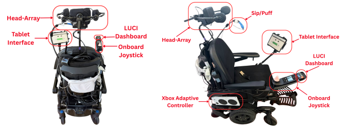
Fig. 3. Our robotic wheelchair—a LUCI Dev Kit, additionally outfitted with a tablet interface and multiple control interfaces (back and side views).
