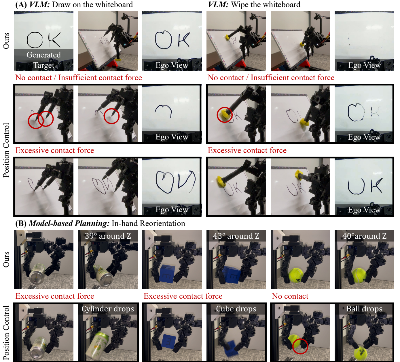
Figure 6: LEAP Hand Results . We show that Minimalist Compliance Control generalizes across embodiments, including dexterous manipulation. We evaluate two high-level strategies: a VLM-based policy for multi-finger drawing and wiping on a whiteboard, and model-based planning for in-hand reorientation of various objects. Both tasks demand precise contact force regulation. Each also includes a position-control baseline, which fails due to contact loss, insufficient force, or excessive force.
