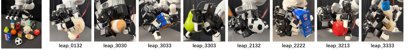
(a) Object list (b) Zero-shot (left four) and trained (right four) grasping results with different LEAP Hand variants.
