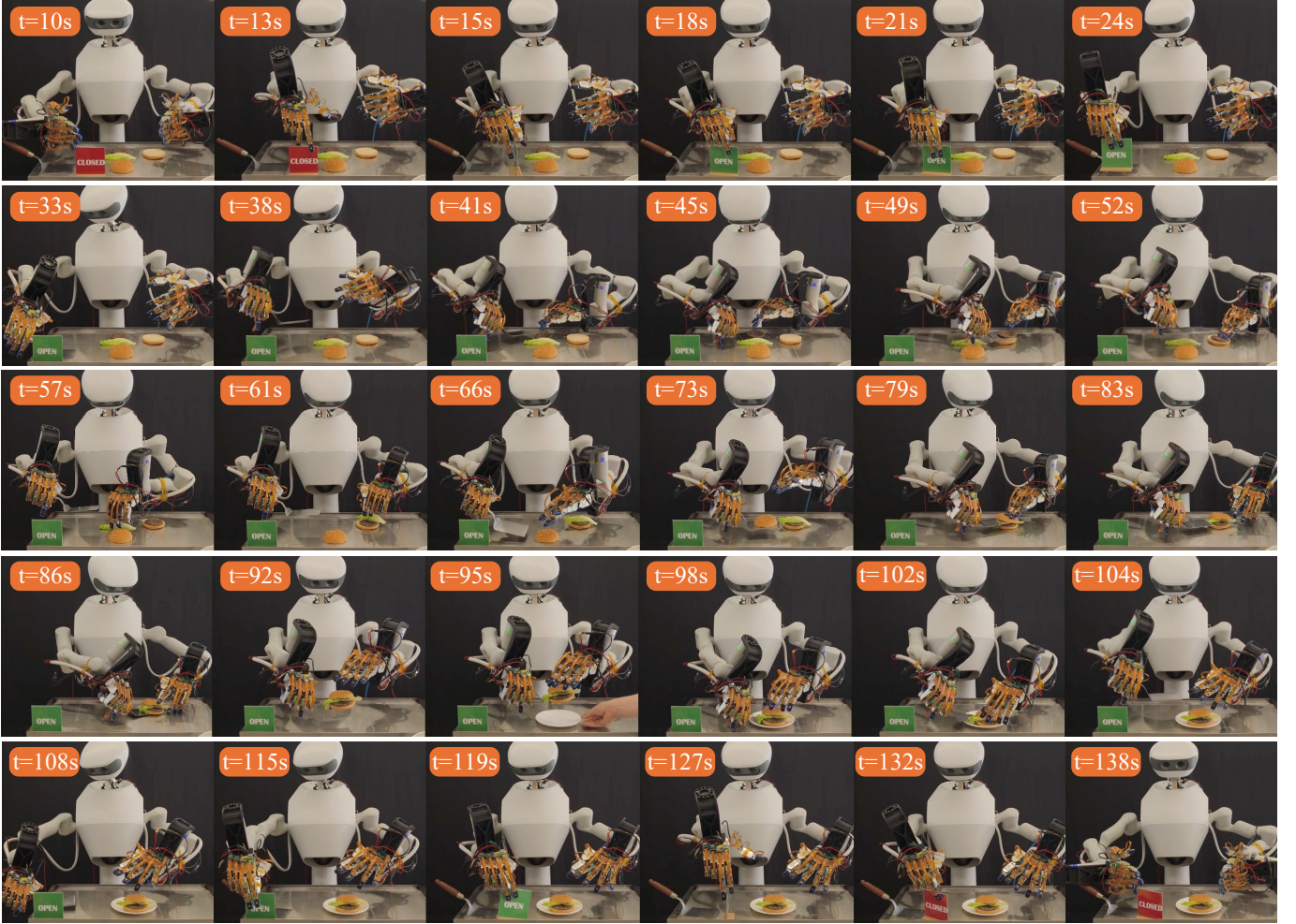
Fig. 5. Successful model rollout on long-horizon task, i.e., making hamburger. We show the successful model rollout with keyframes in 11 stages. The first row represents the robot hand turning the brand to "open". The second row represents the robot hand shoveling meat to bread. The third row represents the robot hand assembling the hamburger. The fourth row represents the robot hand handing over the hamburger to the plate. The fifth row represents the robot hand turning the brand to "close".
