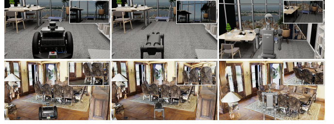
Fig. 3: Cross-embodiment navigation across diverse environments. Each row shows a different robot morphology (Carter, Aliengo, H1); each column shows a different environment source (synthetic, Matterport3D). Insets display egocentric RGB observations, highlighting viewpoint variations across embodiments.
