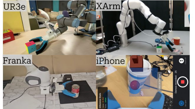
Fig. 7: Cross-embodiment deployment of CAP on a Franka FR3, XArm 6, Universal Robotics UR3e, and an iPhone app. For the robots, the same CAP checkpoint generates EE-space motion that we translate to joint position control with IK. For the iPhone, the user is prompted to move the iPhone to where the robot should go next.
