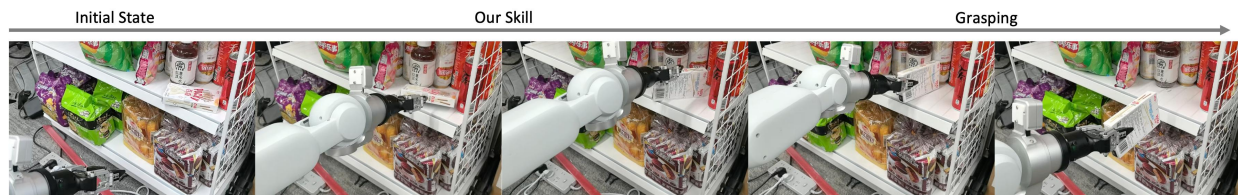
Fig. 10: Humanoid grocery retrieval using extrinsic dexterity. Our policy enables the Galbot G1 to manipulate objects in cluttered shelves by sliding and reorienting them into graspable configurations
