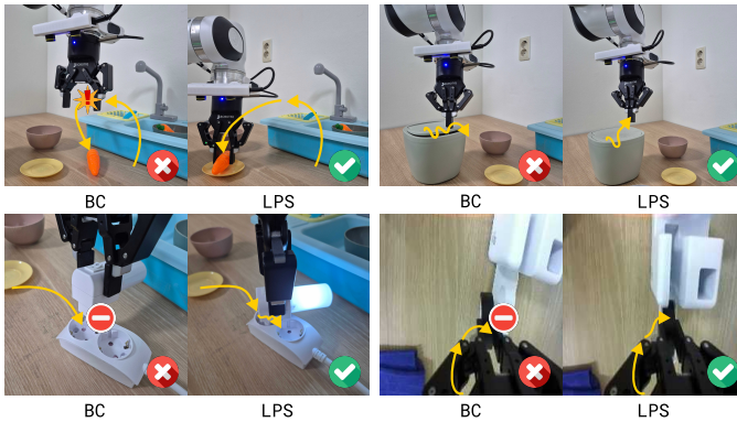
Fig. 9: Qualitative failure modes and corrections. Teleoperation artifacts can induce failures such as premature release ( top-left ), repetitive loops ( top-right ), and freezing during alignment ( bottom ). LPS reduces these failures by selecting higher-value actions at critical decision points.
