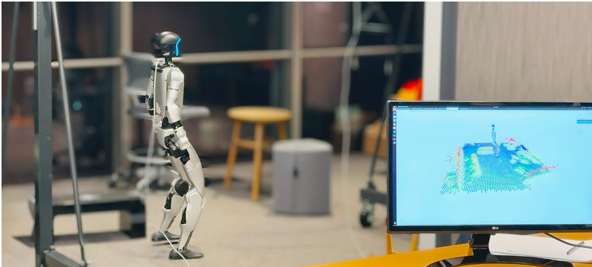
Fig. 2: Real-time visualization for physical robots. Viser enables live debugging of perception and control systems on physical robots. Left: A humanoid robot executing a learned locomotion policy. Right: Visualizing real-time state estimation and mapping in Viser. Viser’s web-based architecture simplifies remote monitoring and debugging.
