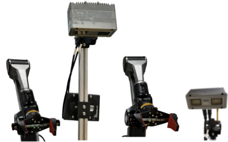
Fig. 6: Overview of the hardware system, consisting of an AgileX CobotMagic dual-arm robot and two industrial binocular stereo cameras.
