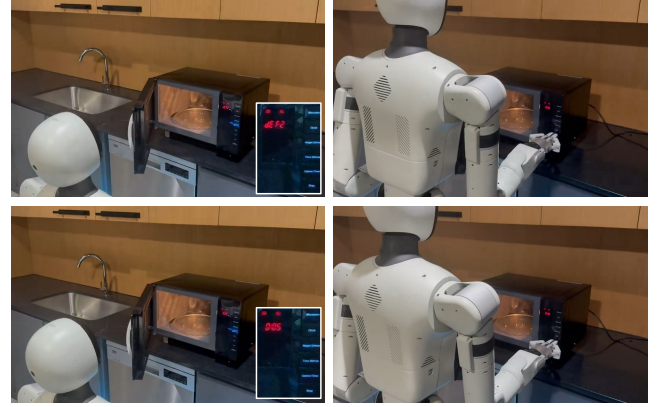
Fig. 13. Demonstration of a robot discovering microwave button functions through interaction.
