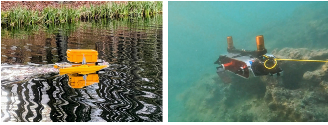
Fig. 2: An autonomous surface vehicle (ASV) and an autonomous underwater vehicle (AUV) mapping bathymetry during our field trials.
