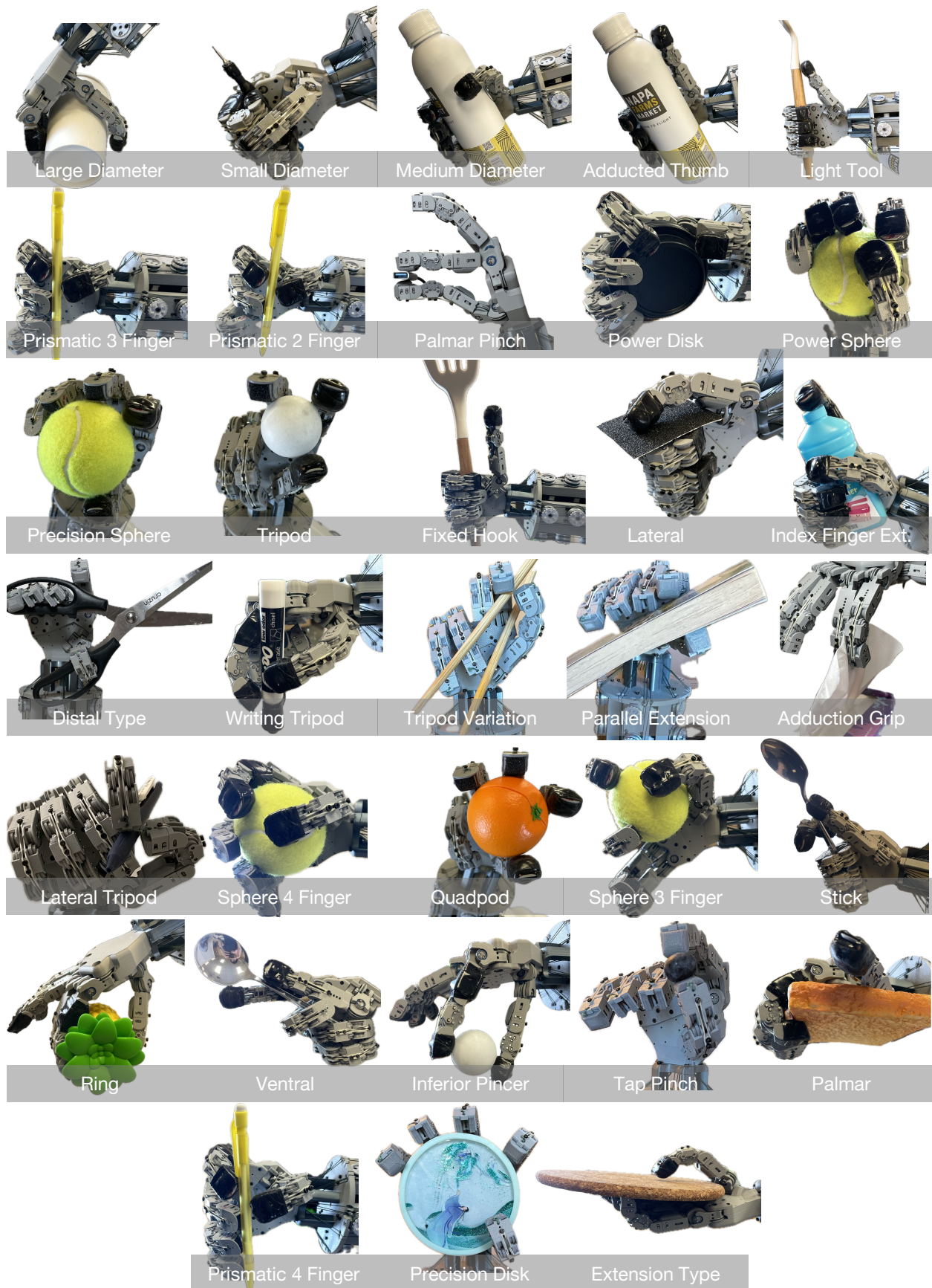
Fig. 11: Grasp Taxonomy Validation. CRAFT demonstrating 33 distinct grasp types from the Feix taxonomy [9]. The hand successfully executes a wide range of configurations, including power grasps (e.g., Large Diameter), precision grasps (e.g., Prismatic Pinch), and intermediate poses, confirming that the compliant design maintains the kinematic versatility required for general-purpose manipulation.
