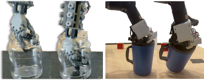
Fig. 14: Narrow Space Accessibility. CRAFT demonstrates the ability to fit into a narrow jar, while the bulkier Leap Hand V2 fails to enter the same workspace due to its rigid linkage size. Both cans have the same radius. Results reproduced with the help of the authors of Leap Hand V2 [33]; reproduced in two labs with different cans.
