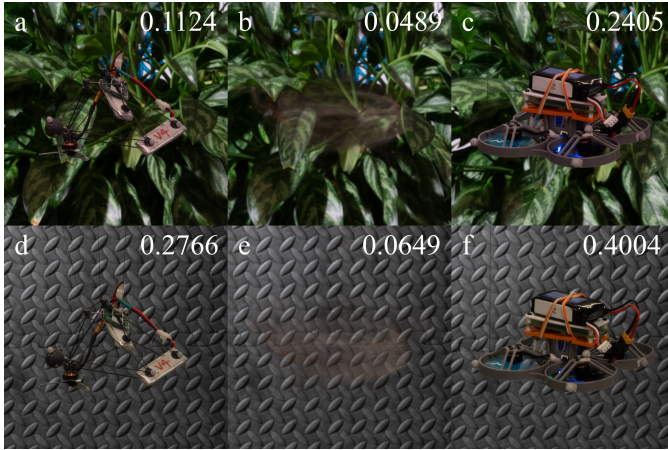
Fig. 8. Comparison of visibility. Three columns show static optimized Phantom Twist (a,d), dynamic hovering optimized Phantom Twist (b,e), and a static quadcopter in front of the same background (c,f). Images in the same row are captured with the same background and the same camera parameters. The number on the right upper corner of each image is the LPIPS score between that image and its corresponding background.
