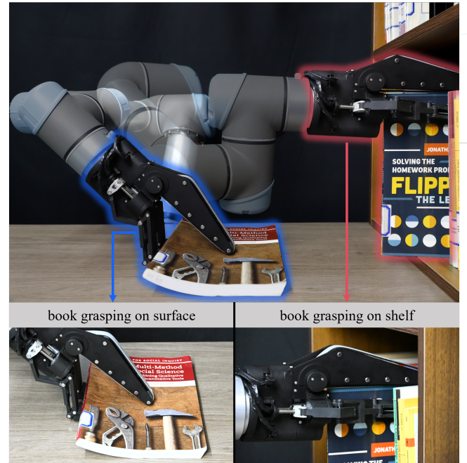
Fig. 1: Grasping demonstration. The gripper grasps books lying flat on the desktop and arranged on the bookshelf, respectively.
