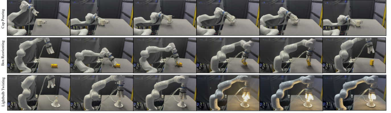
Fig. 7: Real-World Manipulation Results. Sequential frames showing zero-shot real-world execution of contact-rich manipulation tasks with SoftAct , including paper cup pouring, box reorientation, and light bulb screwing. These tasks are challenging as they require compliant manipulation for contact-rich interaction. The robot successfully maintains stable contact and executes task-relevant object motion despite severe embodiment mismatch between the human demonstrator and the non-anthropomorphic soft robot hand.
