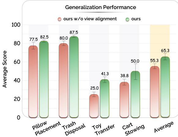
Fig. 8: View alignment ablation. View alignment is essential for effective human-robot co-training, especially for tasks involving variable object heights such as Toy Transfer.
