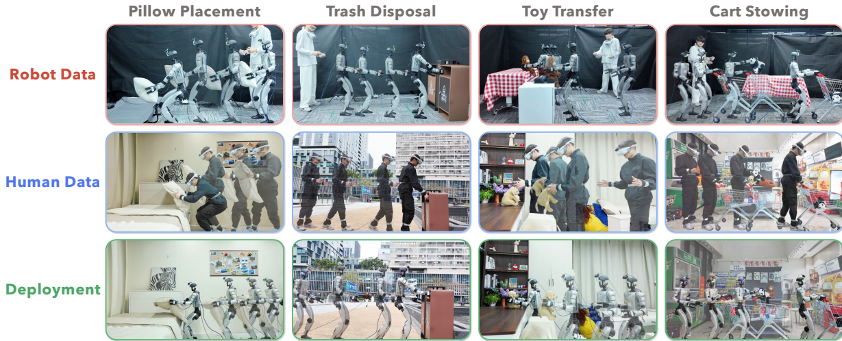
Fig. 4: Humanoid loco-manipulation tasks for evaluation. We design four tasks which span varying levels of difficulty for large-space movement and dexterous manipulation. Robots are teleoperated in laboratories as the source domain ( Top ). Human-centric scenes occur in human demonstrations only ( Middle ), and set as testbeds for generalization evaluation ( Bottom ).
